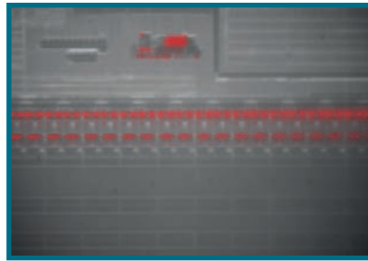
Overlay of the photo-emission results on IR vision of the chip.
